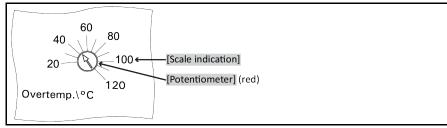
The overtemperature protection is installed only in temperature control units that have a heater. The flow temperature is monitored to ensure the safety of your system. It is set immediately after you have filled the system with thermal fluid.
