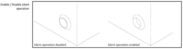
Enabling silent operation on the temperature control unit reduces the noise level by decreasing the pump capacity. For the exact position of the switch >**Change pump speed**< [114] please refer to the "Wiring diagram".  $\rightarrow$  From page 59, section **»Annex**«.
