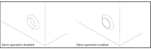
Enabling silent operation on the temperature control unit reduces the noise level by decreasing the pump capacity. For the exact position of the switch >Change pump speed< [114] please refer to the "Wiring diagram". → From page 55, section »Annex«.
