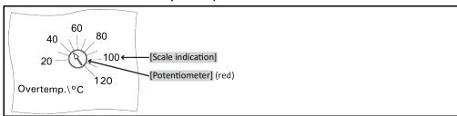
The overtemperature protection is installed only in temperature control units that have a heater. The flow temperature is monitored to ensure the safety of your system. It is set immediately after you have filled the system with thermal fluid.
