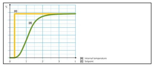
Internal, dynamic temperature control with possible overshooting of the temperature
