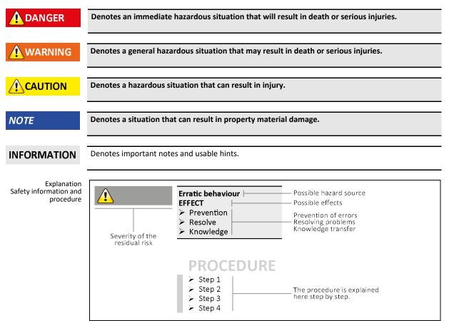
The safety information in this manual is designed to protect the responsible body, operator and the equipment from damage. Safety instructions appear at the beginning of each chapter and before instructions. First inform yourself about any residual risks due to misuse before you start an operation.
